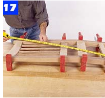
Join the back rail and slats to the legs. Apply the glue sparingly, clamp, and check that the diagonals are equal.
