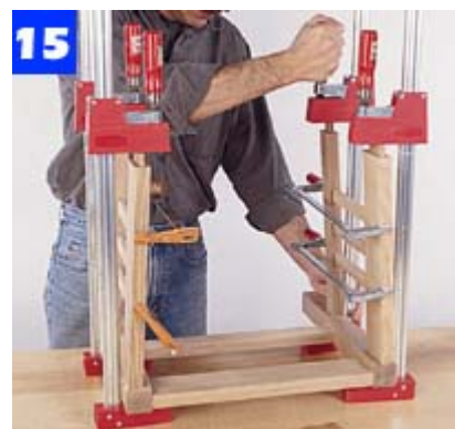
Spread glue on the rail and leg mating surfaces. Join the side rails to the front leg assembly and clamp.
