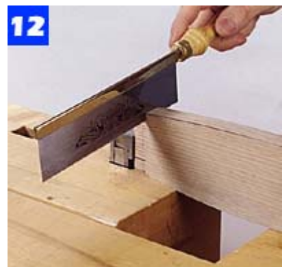
Cut the shoulders of the curved back rail tenons with a small backsaw. First cut in from the end, then across the grain.
