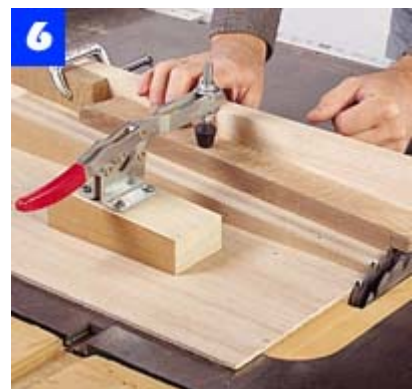
To cut the angled tenons on the side rails, support the stock in a table saw jig that holds the work at a 4° angle.
