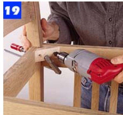
Use a clamp to hold the corner blocks in position as you bore and countersink pilot holes for fastening to the rails.
