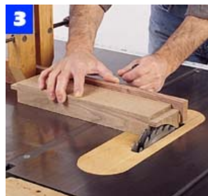
Use a table saw and dado blade to cut the tenons in the blanks for the curved back rails. These tenons are not centered.
