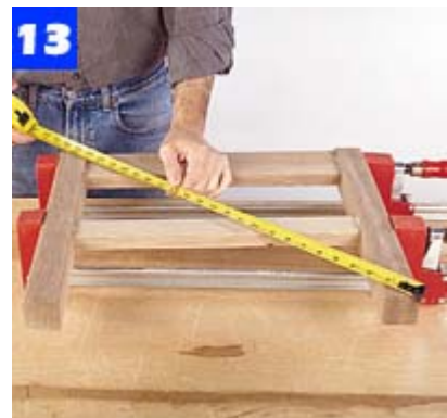
Join the front rails to the legs, and clamp. Compare opposite diagonal measurements to check for square.
