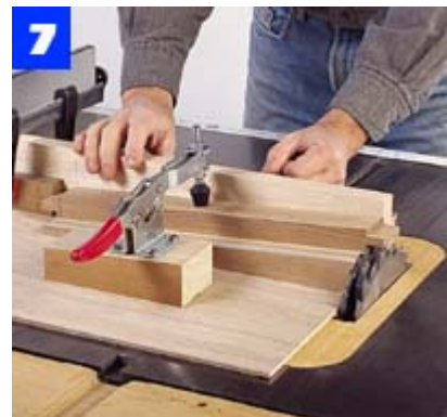
When cutting the opposite tenon faces on the rails, reverse the ramp on the jig and readjust the dado blade height.
