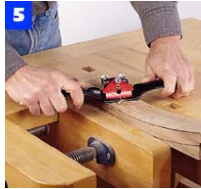
Use a spokeshave to smooth the inside curve of the back rail, and then cut and smooth the outer curve.
