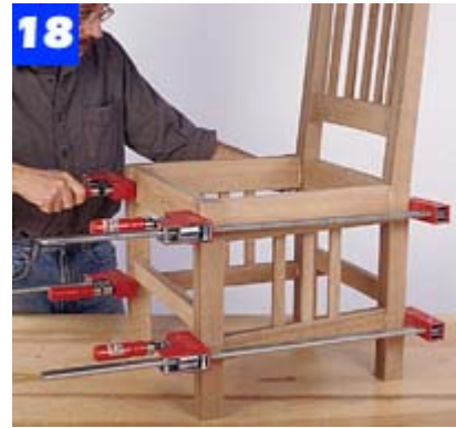
Join the back subassembly to the front-leg/side-rail assembly. Work on a flat surface so the legs remain even.
