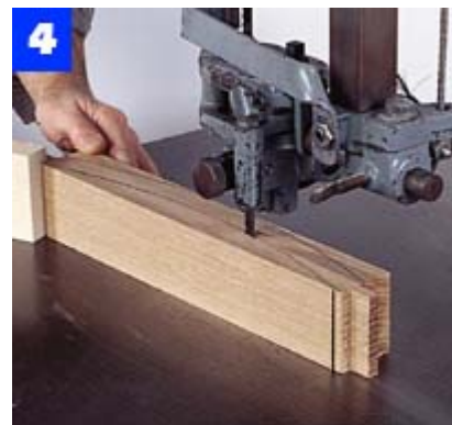
Lay out the back-rail curve onto the edge of each rail blank. Then, cut the inside curve on the band saw.
