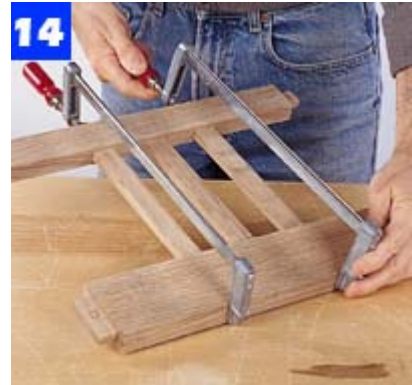
Join the side slats to the rails. It's not necessary to use glue since the slats are held captive between the rails.
