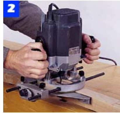
Mark the mortise locations in the chair legs, and use a plunge router with an edge guide to cut the mortises.
