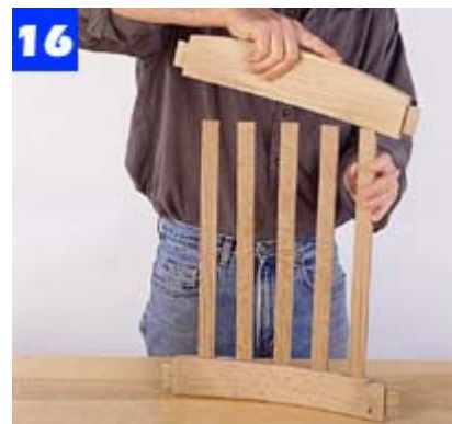
Join the back slats to the curved rails. If a slat is too loose in its mortise, add a drop of glue to keep it from rattling.
