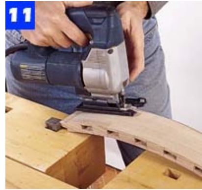
Use a template to lay out the arched profile of the upper back rail. Then, cut to the line with a sabre saw and smooth.
